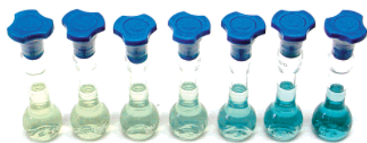
Figure 2. Solution of 1 (concentration = 1.47 \times 10^{-4} M) in acetonitrile/diethyl ether mixture demonstrating the remarkable color changes. Diethyl ether composition (from left to right): 64, 68, 72, 74, 76, 78, 80%.
